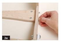
2. Working from the outside, insert the non-gear ends of the warp and cloth beams through the holes in the right side of the loom, then into the holes in the left side of the loom. Place a fender washer on each 1" screw and secure the warp and cloth beams on the left side of the loom. (Photo 3) Flip the ratchet dogs over so they sit on top of the gears.
