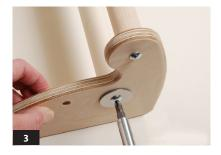
3. Insert and center the handles into the holes in the ends of the warp and cloth beams. If the dowels are a tight fit, use a hammer to gently tap them into place. Use the 3/8" screws to secure the handles. You can rub a bit of bar soap or paste wax on the screw threads to make them easier to turn, or use an electric screwdriver if you have one (Photos 4–5 on next page).
