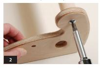
15" Looms: Align the center cross brace with the pairs of holes in the loom sides. Place a barrel nut into one of the holes in the brace with the slot on top and parallel to the long sides of the brace. Insert a 2" bolt through the loom side and screw into the barrel nut. Repeat for the remaining holes in the cross brace. (Photo 2a)
