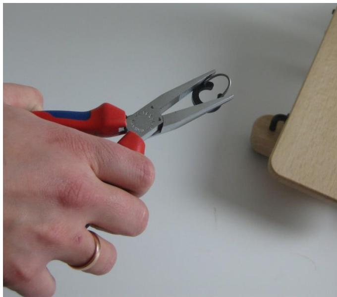
If the yarn guide becomes too easy to slide on the flyer arms, you can use a pair of pliers to tighten the guide, pushing it together where the metal wire enters the plastic part.
