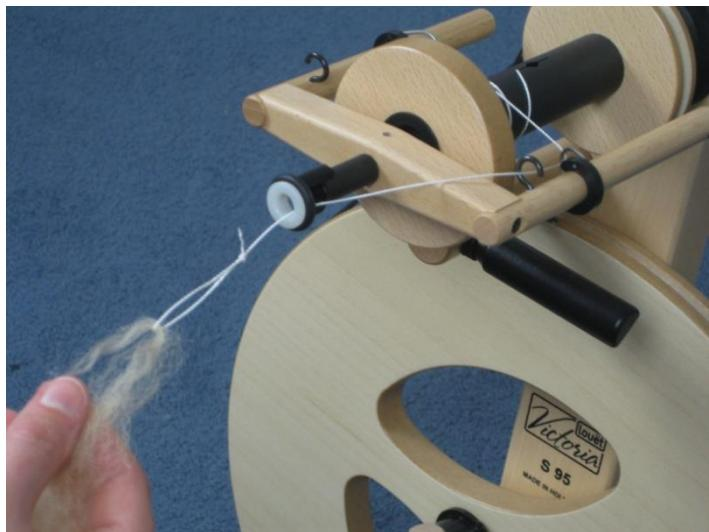
Guide a starter yarn through the orifice, around the hook and through the yarn guide slide. It does not matter which side of the flyer you use. Make a double knot at the very end of the yarn and insert it into the slot of the bobbin core. Move the yarn guide to a location where it will pull the yarn in a direction the slot will hold the knot.
