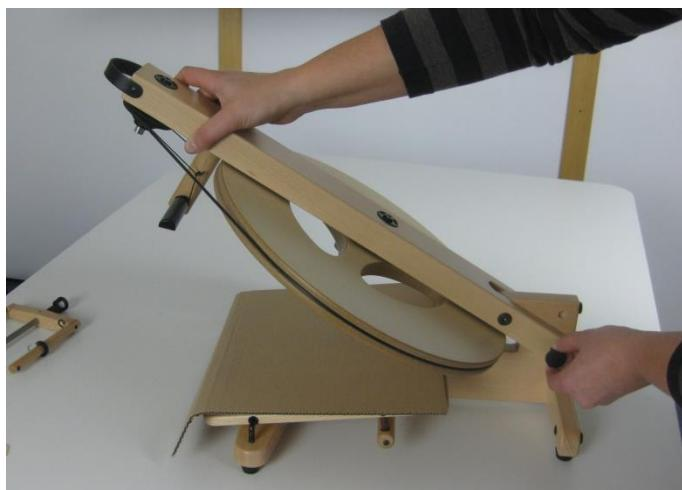
Place the wheel flat on the table. Pull the black knob and lift the back post up. You can release the knob after you start to lift the post and it will automatically lock in place once the post is in its proper upright position.
