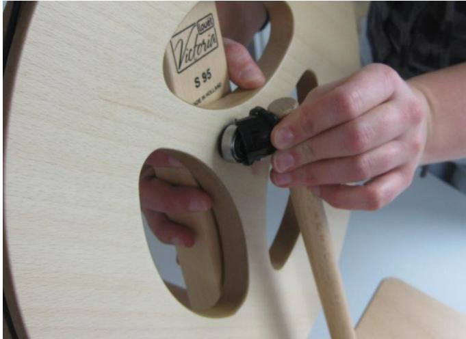
Place the cup on the footman over the ball bearing of the wheel and push the locking ring forward against the rim on the cup. If you position the cup at an angle to the bearing, while pushing it on, the cup snaps on easier. When you need to remove the cup again, retract the locking ring and then twist the footman, allowing the cup to snap off of the bearing easily.
