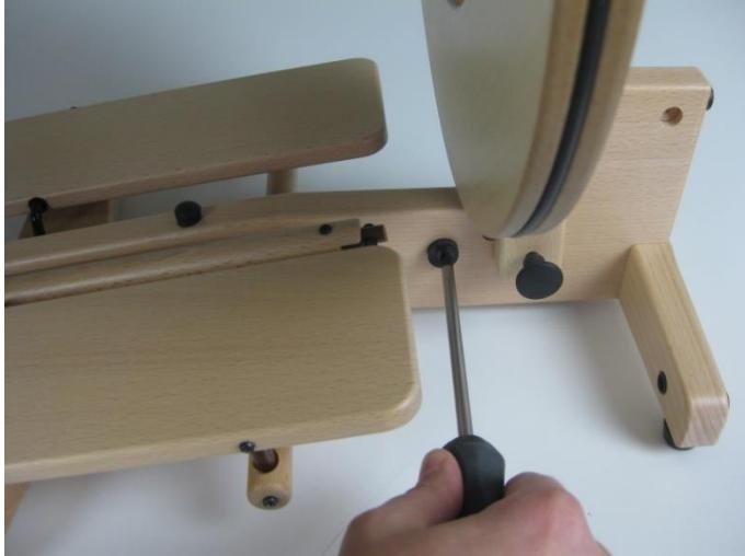
If it happens that some play arises in the locking system of the post, it can be repaired by adjusting the buffer. Release the screw of the buffer and turn it to a position so that it pushes the bottom of the post slightly backwards. The locking knob should fall inside just when the post hits the buffer. Fasten the screw after the buffer is turned into its proper position.
