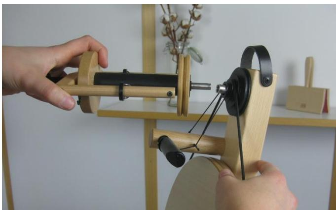
Slide the flyer shaft through the bobbin, from the side of the bobbin where there is no groove in the bobbin rim.
